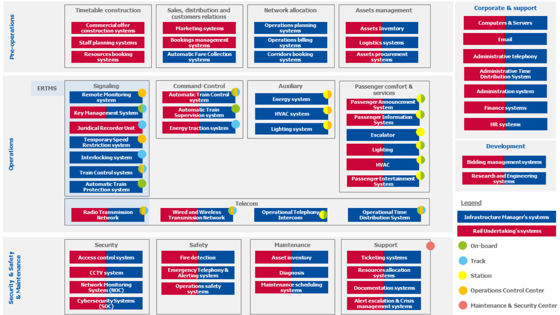
Figure Note: Background colours indicate the actor who is usually in charge of the system (this could vary according to the organisation or project). A coloured pastille shows the most likely location of the system; some systems have assets in several locations. ERTMS is considered as it is the ATC that is harmonised for EU. The scope of the ERTMS is depicted with a light blue colour, covering Signalling and Radio systems.
